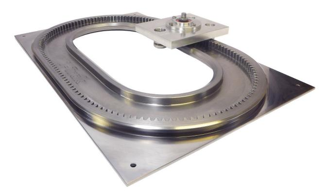
The gear teeth on the track are precision machined and surface hardened to produce outstanding strength and durability. When used with a hardened pinion and properly lubricated, high driving forces, minimal backlash and long life will be achieved.
