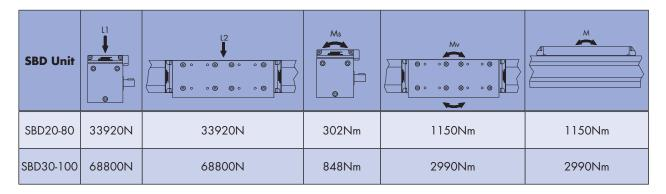
The table below includes the parameters necessary to calculate the performance and duty of an SBD system.
