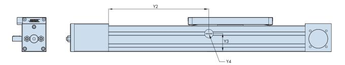
Re-lubrication of the ball guide carriage block is via an access point in the side of the beam (see above), which is closed off with a threaded plug. The lubrication interval depends on the length of stroke, speed and duty. For further details regarding lubrication procedures please contact Hepco's technical department.
